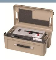
The test lamp LE3 is used to test the function of all flame detectors over distances up to 10 m. It is housed in a transportable case together with the required accessories. In addition, the case enables the test lamp to be kept in a dust-free condition.
